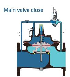
When the upstream pressure drops below the pilot valve's set pressure, the pilot valve closes, allowing water to enter the upper bonnet chamber of the main valve and forcing the main valve to shut.
