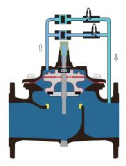
When the pump is started, the main valve drains water from the bonnet chamber, and the main valve first opens slowly and then quickly.
