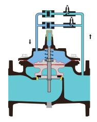
When the pump is stopped, water enters the bonnet chamber on the main valve, and the main valve closes quickly and then slowly.
